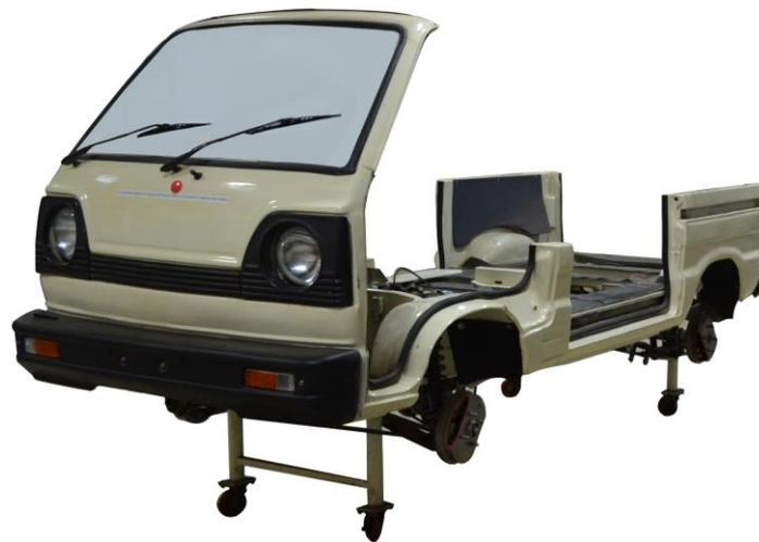
In the automotive sub-systems component, the students will be introduced to multiple functional cut sections and working standalone demonstrators of automobile sub-assemblies. Also, a few important aggregates like engine, clutch, and the gearbox will be dismantled, to study their construction features and assembled back by the students. The topics covered in this component are:
