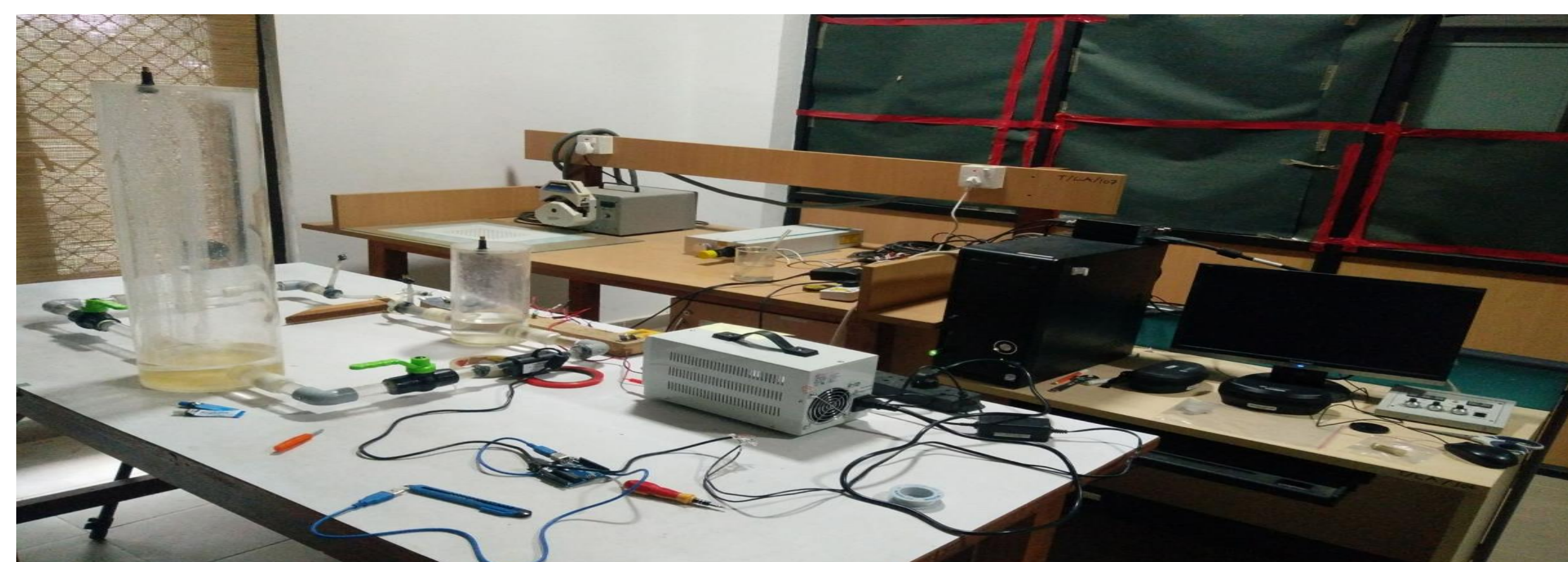
Fig. Particle image velocimetry on systemic mock circulation loop The image shows a systemic mock circulation loop which is used to test an inhouse developed percutaneous type left ventricular assist device, on which piv is being done to test the flow field.
