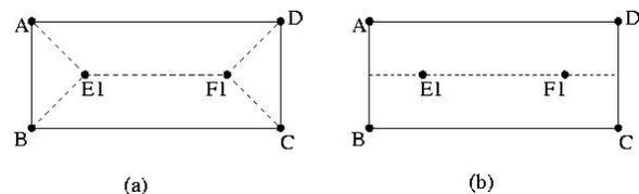
Fig. 1. Medial Axis and Mid-curve.
