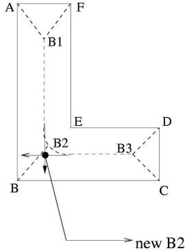
Fig. 3. Replacing MAT at a concave corner.
