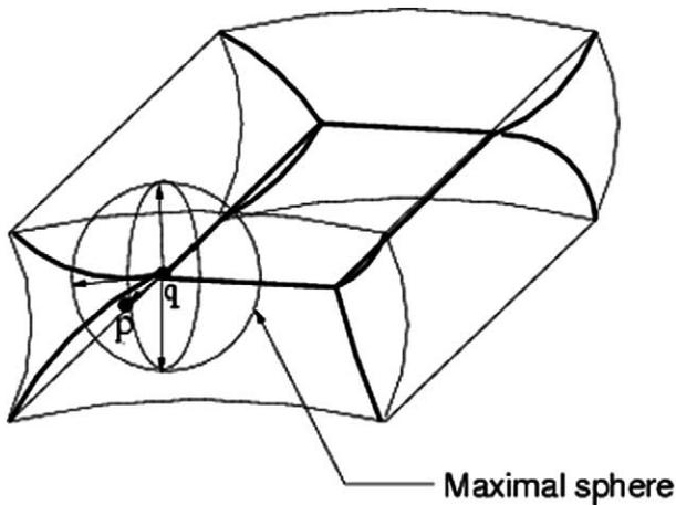
Fig. 1. Boundary and its medial axis.
