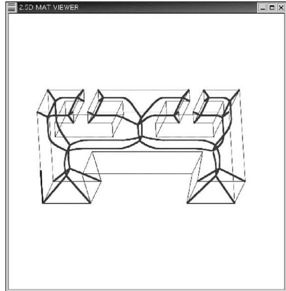
Fig. 20. MAT of a machine tool bed.
