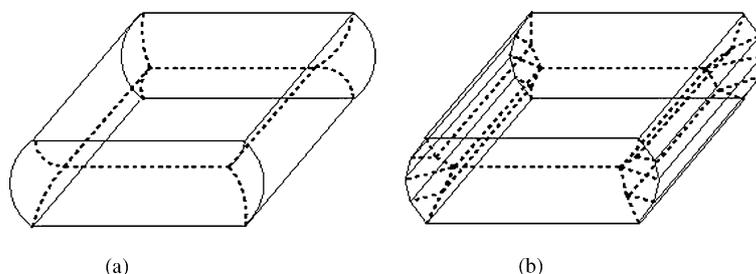
Fig. 2. Effect of discretising boundary on MAT.
