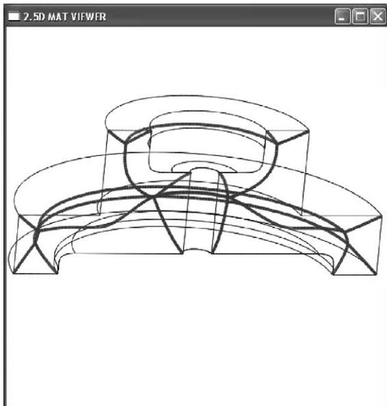
Fig. 23. MAT of a bearing housing.
