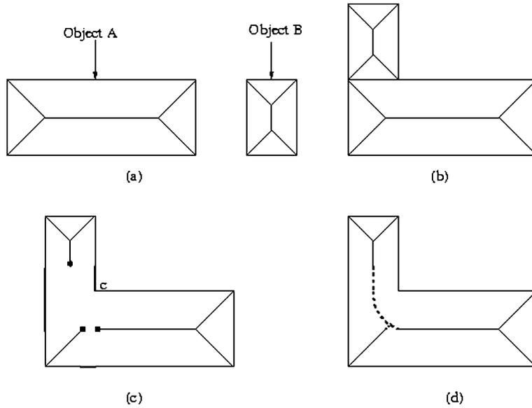
Fig. 27. Medial axis for union of objects.
