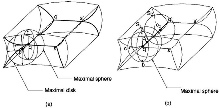
Fig. 15. Seam between junction points.
