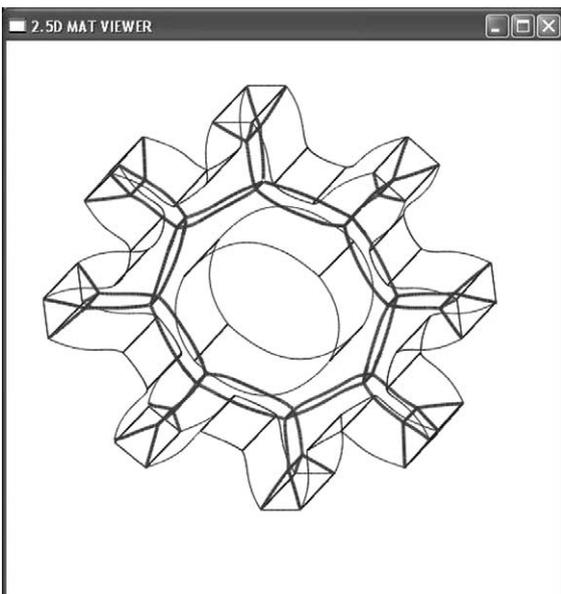
Fig. 19. MAT of gear wheel.
