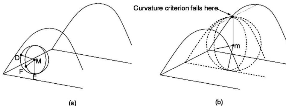
Fig. 9. Curvature criterion.
