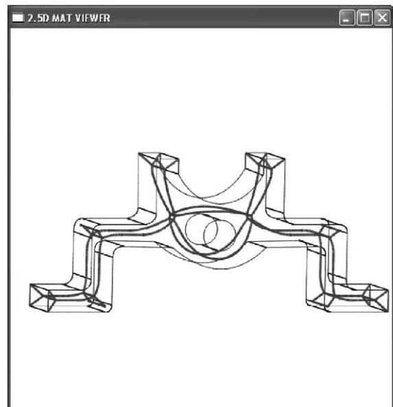
Fig. 21. MAT of a housing bracket.
