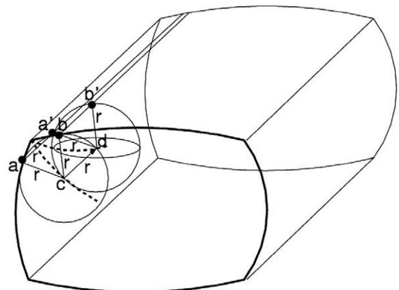
Fig. 13. Seam points using normal points for extruded objects.
