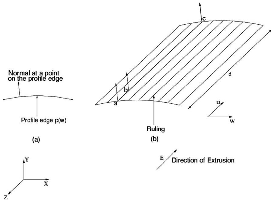
Fig. 4. Normal vector on extruded face.
