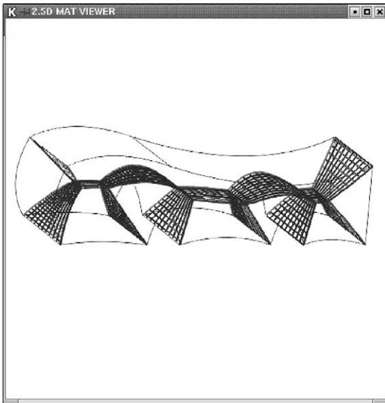
Fig. 25. Mesh of iso-parametric curves on some MAT patches for the test object in Fig. 6.
