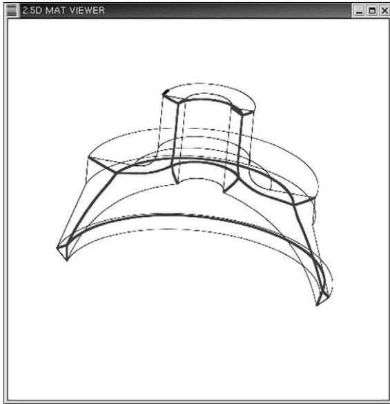
Fig. 22. MAT of universal spider joint.
