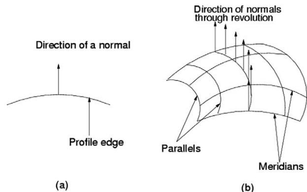
Fig. 5. Normals at the surface of revolution.
