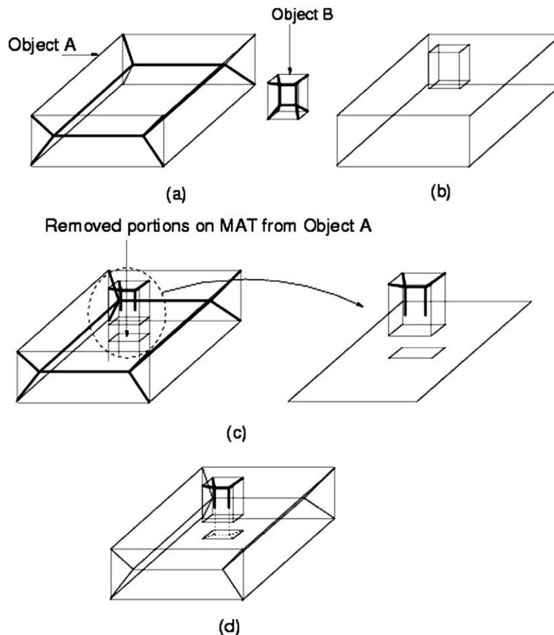
Fig. 26. Medial axis for union of two 3D objects.
