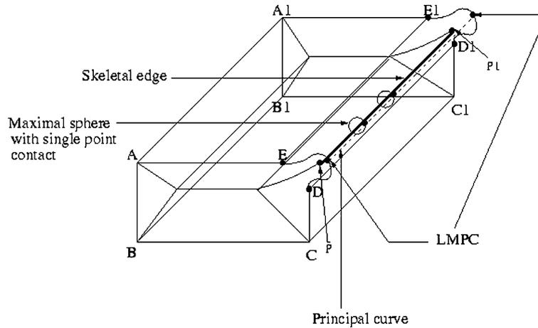
Fig. 14. Smooth case and violation of curvature criterion.
