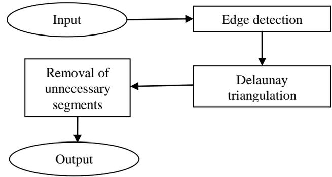
**Fig 2: Framework for the generation of medial**
