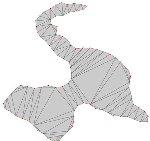
**Fig 3: Delaunay triangulated boundary**
